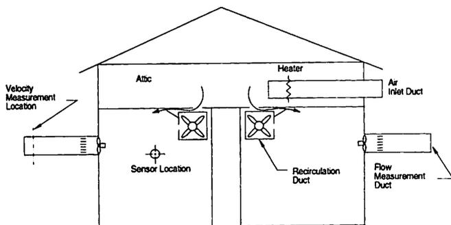
Fig. 3. Cross sectional schematic of experimental units.
