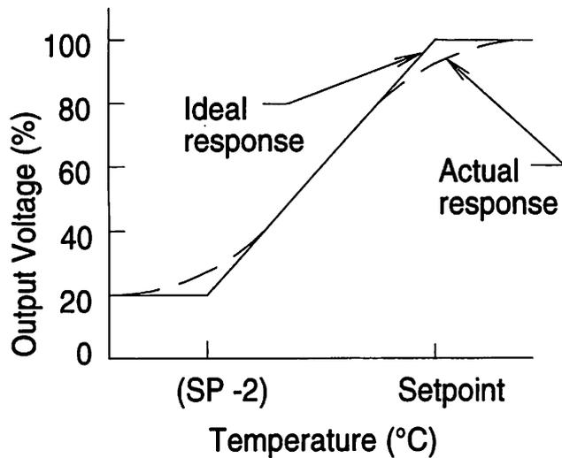
Fig. 1. Controller characteristic curve (fan-on mode).
