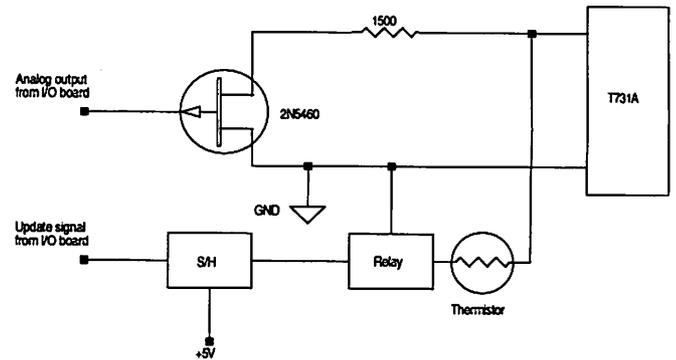
Fig. 2. Thermistor bypass circuit.
