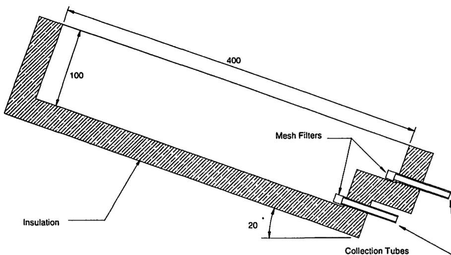
**Fig. 1. Cross-section of a runoff collection tray.**
