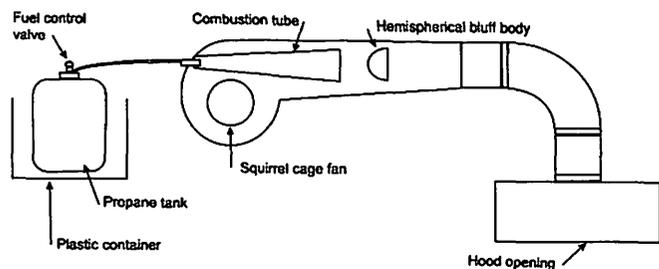
**Fig. 1. Schematic of the prototype.**
