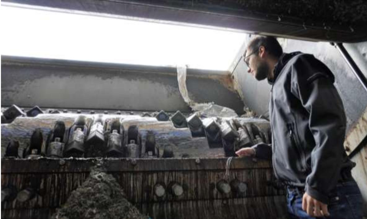
The huge round jaws of the shredder were still hot to the touch, even though the machine had been off for five hours due to routine service work. Shredding is the first step in processing the annual capacity of 35,000 tonnes of films at the recycling plant in Wels.
