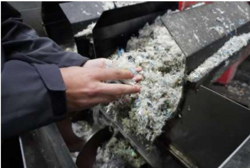
A second shredding is needed to produce the desired small flake. Then comes washing to remove the huge range of contaminants. The keys, stones and euros that the magnet did not remove collect at the bottom of the water tank (yes, that's what happened to your car keys!). The operation here recycles 90% of their water via settling and flocculation. A centrifuge as well as a filter press are needed to remove the
