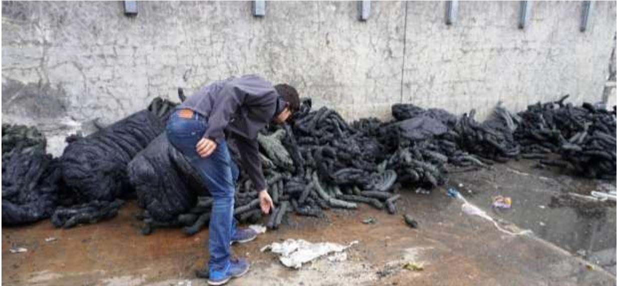
The contaminants are continually removed from the filter and consist of other plastics (PET, PVC) and organic material such as hair, wood etc. None of these things are identifiable because they are encased in grey plastic. The fate of this is the waste to energy furnaces, producing electricity. Glues and label inks produce gases at this temperature and a degassing step is needed also. Additions of colour or plasticizers can be made at this stage through ports in the extruder pipe.
